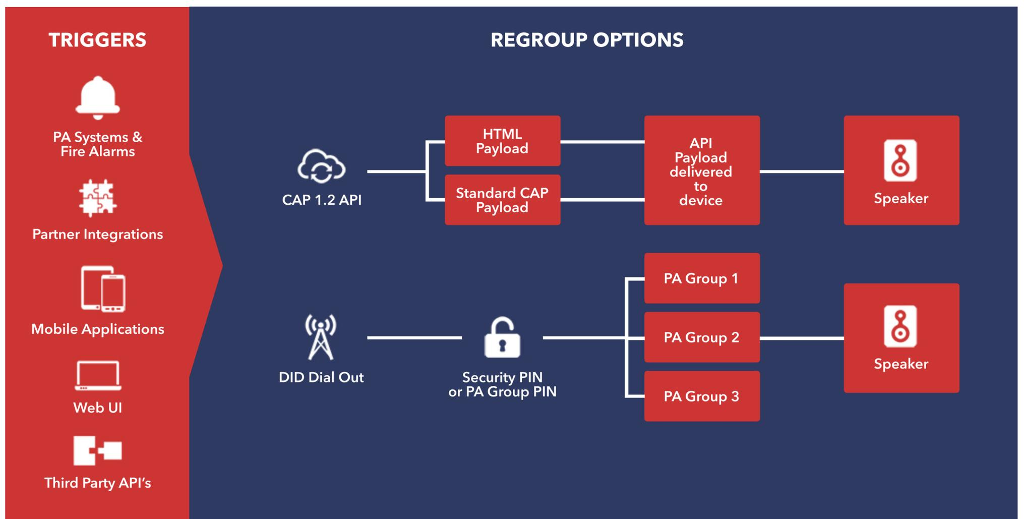
Newer Simplex Fire Panel Models can trigger or receive real-time alerts from Regroup using direct FEMA standard CAP 1.2 APIs.
